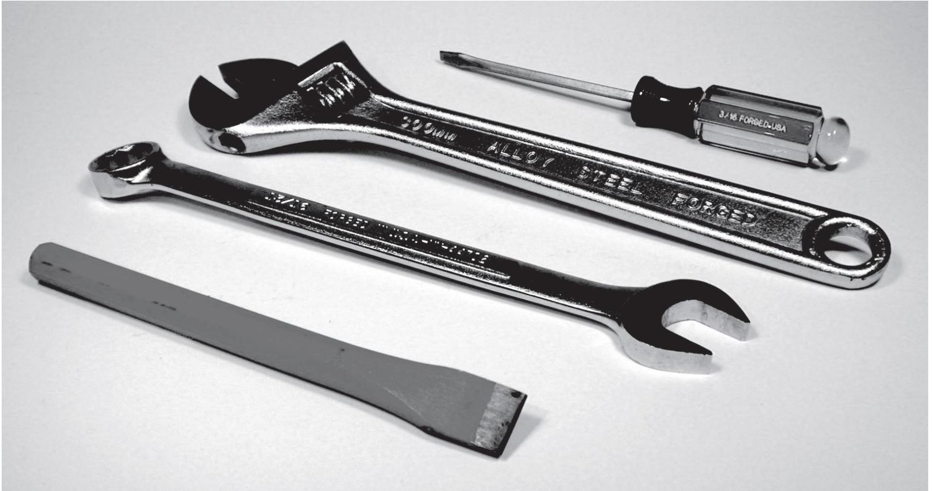
FIGURE 2: Examples of hardware produced by forging.
